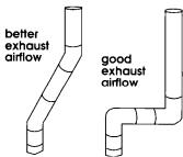
Four-inch metal exhaust duct is required. Plan installation to use the fewest number of elbows and turns.
